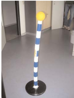
Figure 1. Ball pendulum for stroke simulation.
